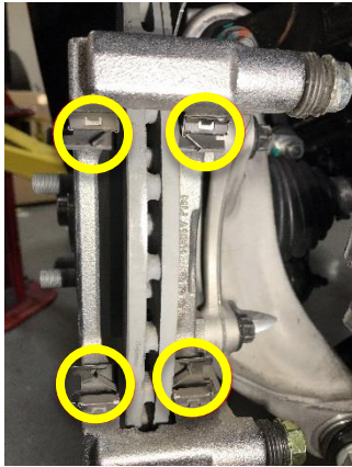
Figure 20 (Model 3 abutment springs)
