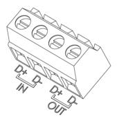
Form a daisy-chained network by connecting the cables from OUT to IN and always from positive to positive and negative to negative between each of the participating Wall Connectors (refer to Example of the Communication Wiring on page 28).
