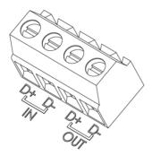
1. Form a daisy-chained network by connecting the cables from OUT to IN and
