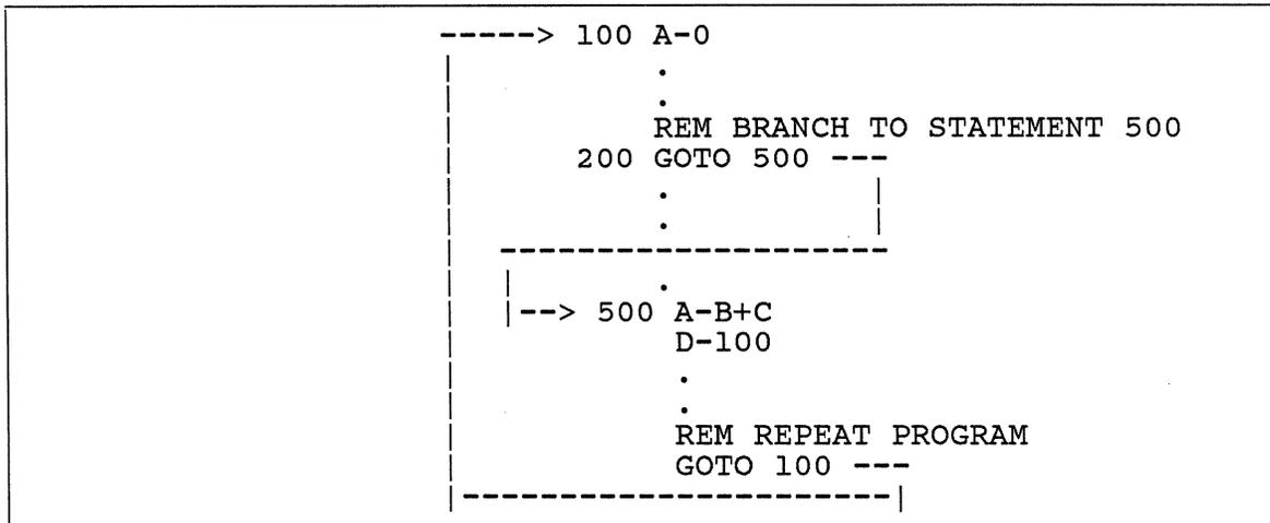
Figure B. Example of Correct Usage of GOTO Statement
