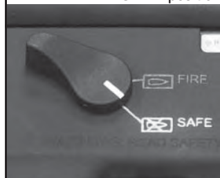
fig. 3 Manual safety in “SAFE” position
