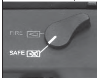
fig. 1 Manual safety in “SAFE” position
