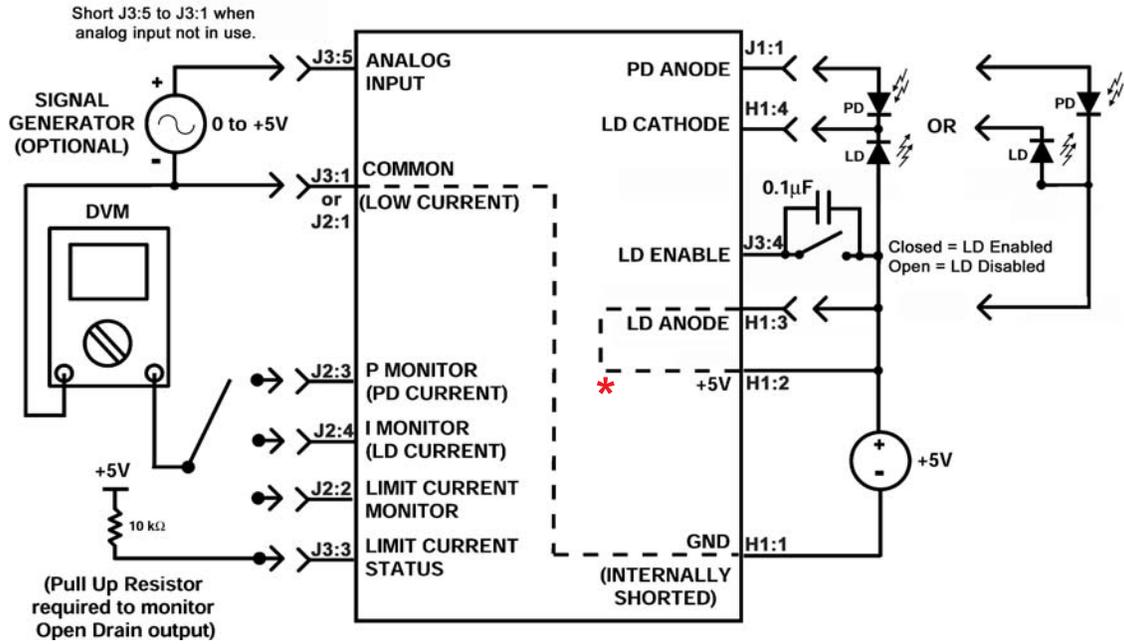
\* Note: In the default configuration, pins 2 and 3 on H1 are jumpered. The PLD10K-CH and PLD5K-CH are shipped in this configuration. Since this jumper makes the connection between these pins, it eliminates the need for the user to connect the pins.
