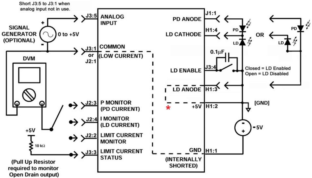
**Typical Setup for Type A or B laser diode - High Compliance Voltage operation\***
