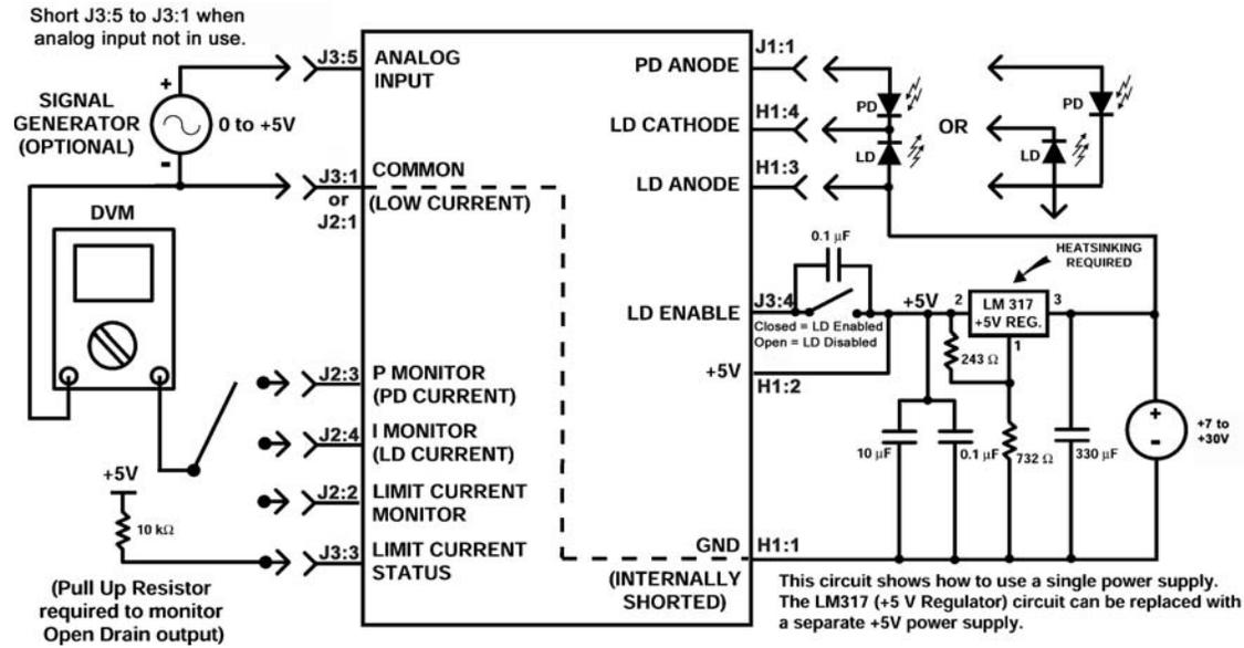
**\*Note:** When configuring the PLD10K-CH and PLD5K-CH for High Compliance operation, the jumper must be cut on Terminal Block H1 between pins 2 and 3. This allows the addition of a separate power supply to the laser diode anode (H1, Pin 3). See the diagram below for the location of the jumper.
