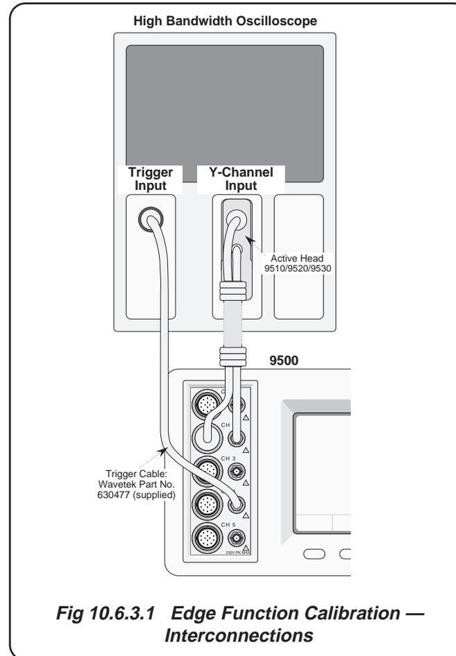
**Fig 10.6.3.1 Edge Function Calibration — Interconnections**
