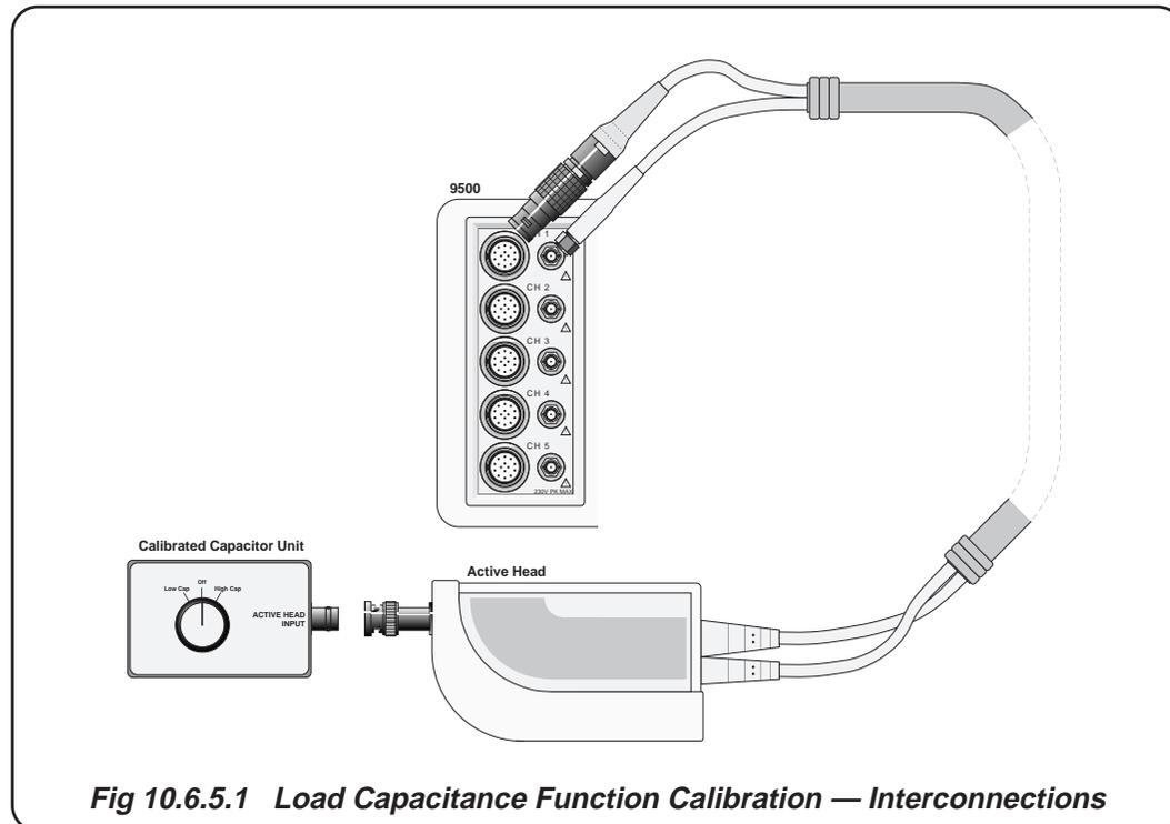
**Fig 10.6.5.1 Load Capacitance Function Calibration — Interconnections**
