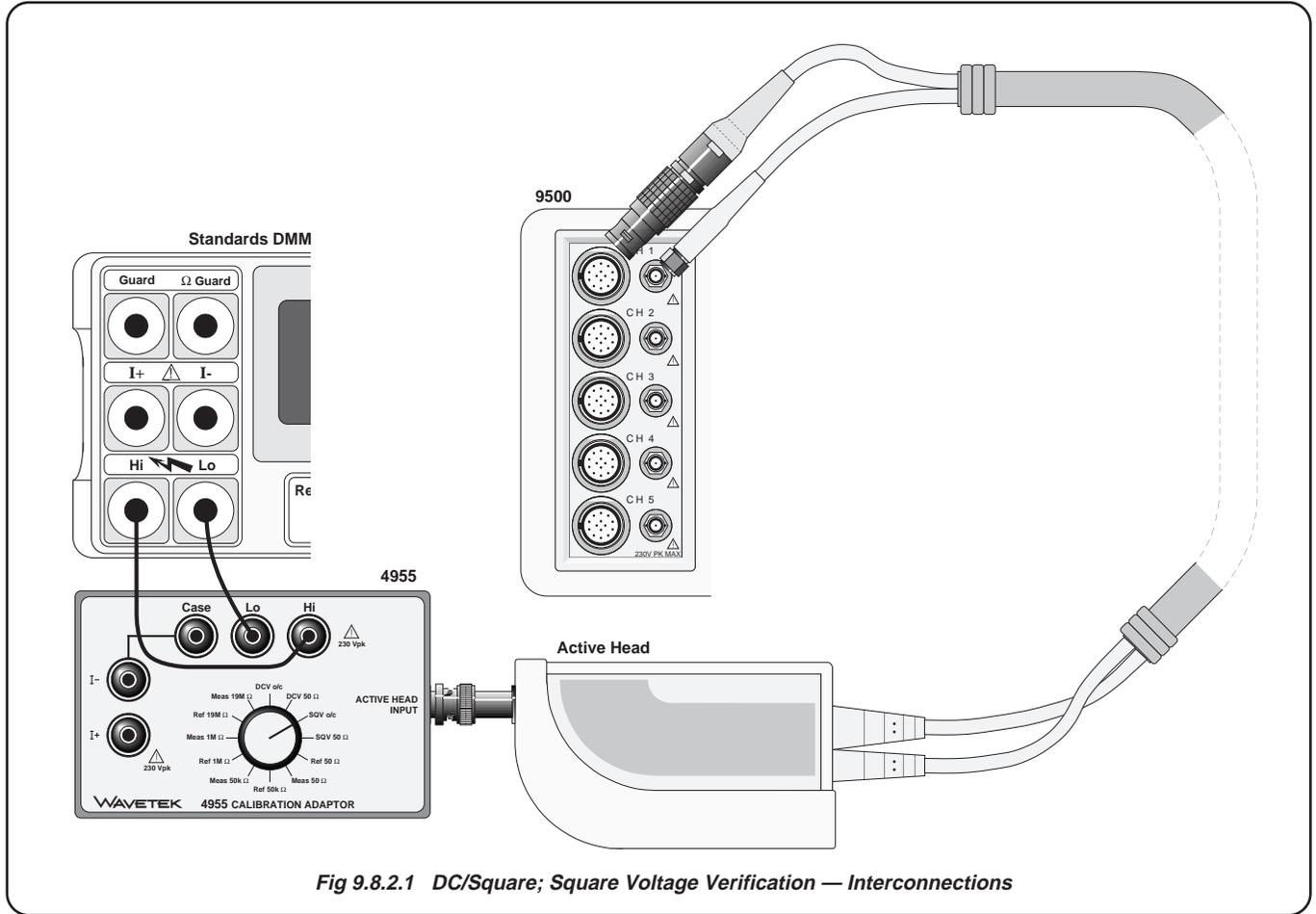
**Fig 9.8.2.1 DC/Square; Square Voltage Verification — Interconnections**
