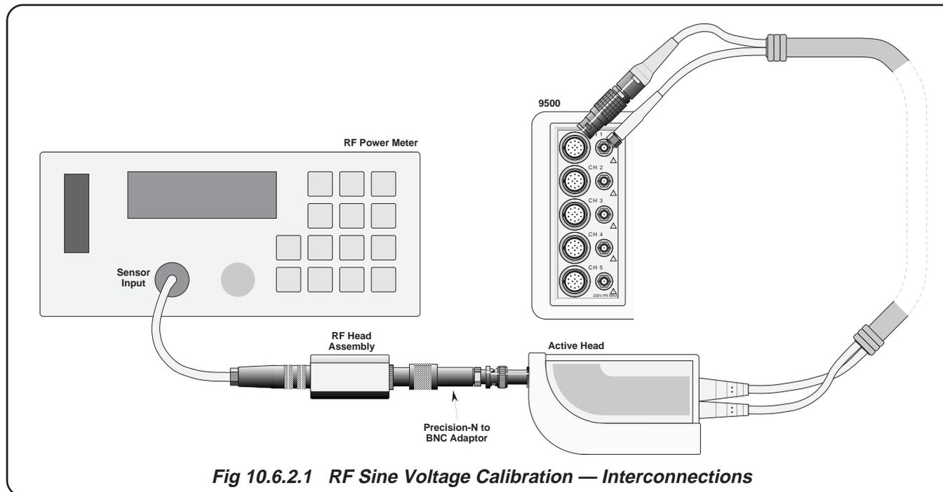
Fig 10.6.2.1 RF Sine Voltage Calibration — Interconnections
