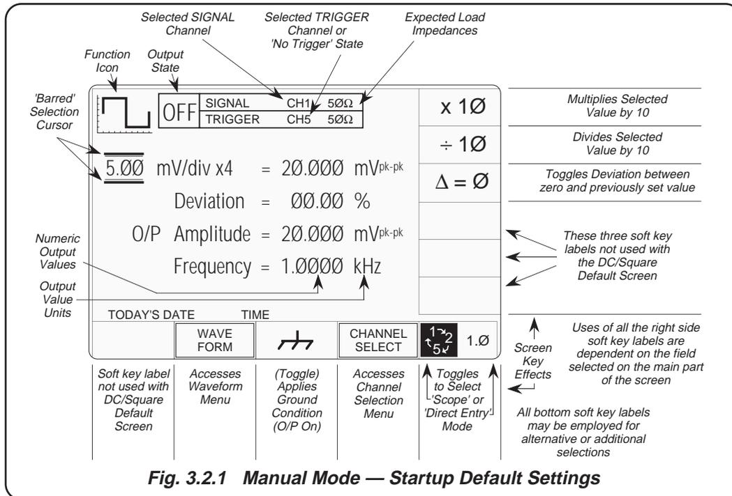
**Fig. 3.2.1 Manual Mode — Startup Default Settings**
