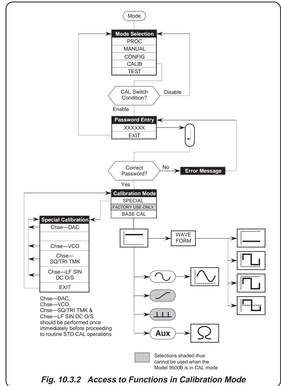
Fig. 10.3.2 Access to Functions in Calibration Mode
