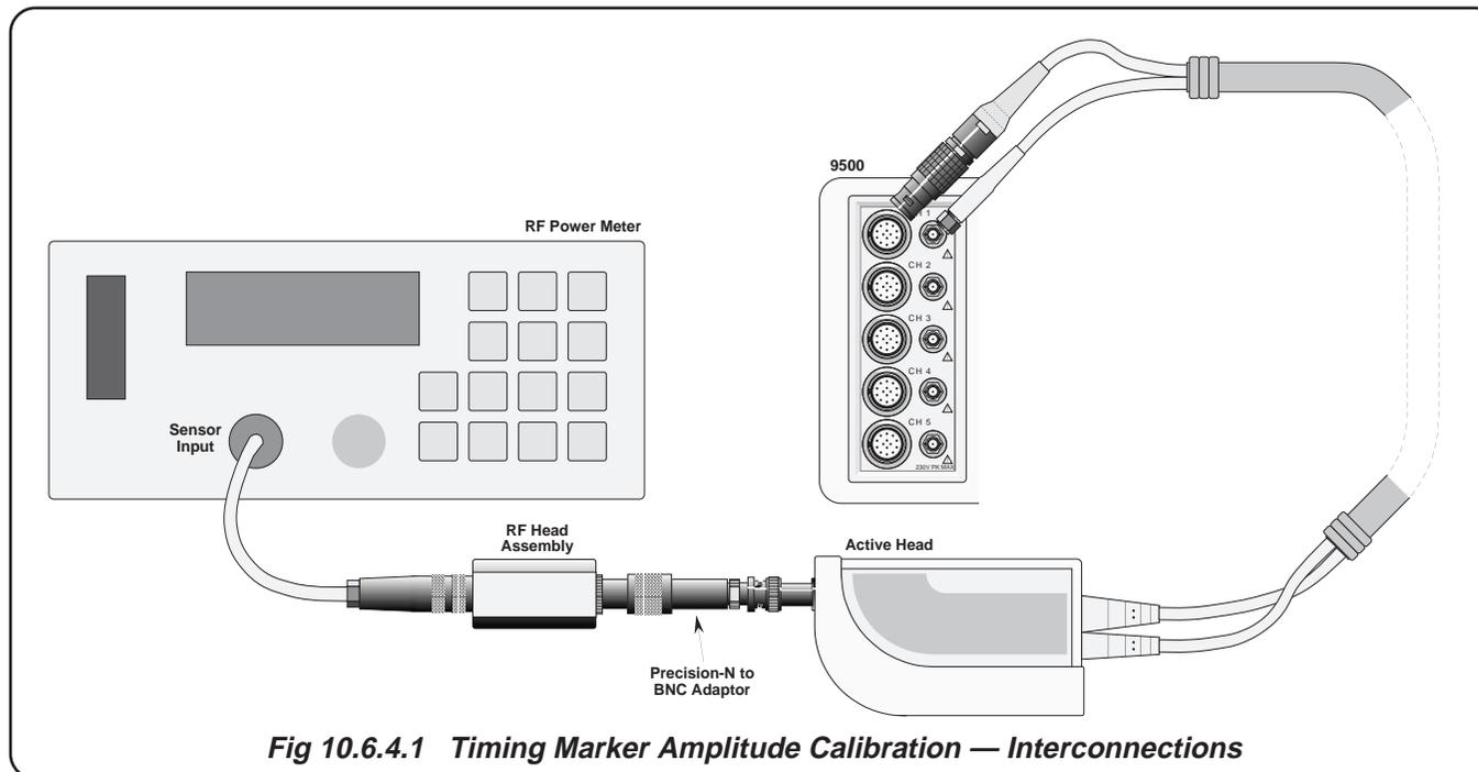
**Fig 10.6.4.1 Timing Marker Amplitude Calibration — Interconnections**
