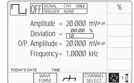
Fig. 4.4.6 Numeric Entry — Effect on Deviation Value and Screen Key Labels
