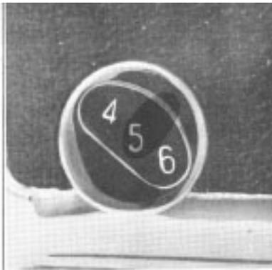
10) Only even numbers will show in the exposure counter window after the number "8" appears. Odd numbers are indicated by a line. (On the Model-E, only even numbers appear after the number "4". Odd numbers are indicated by a dot.)
