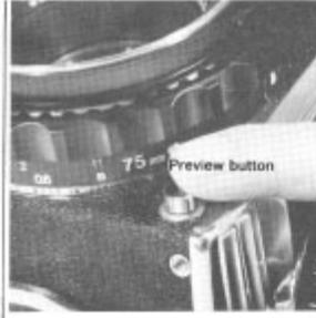
7) All Bronica interchangeable lenses have automatic diaphragm, and critical focusing and viewing can be done with full aperture. Check the depth-of-field or adjust the background vignetting by depressing the preview button.
