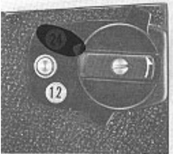
**S2A:** Switch lever may be moved to the 24 exposure position at any time if you have forgotten to do so before loading.
