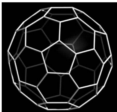
FIGURE 1. A perspective view of the soccer-ball-like structure of buckminsterfullerene C_{60} showing 12 pentagons and 20 hexagons of carbon atoms.
