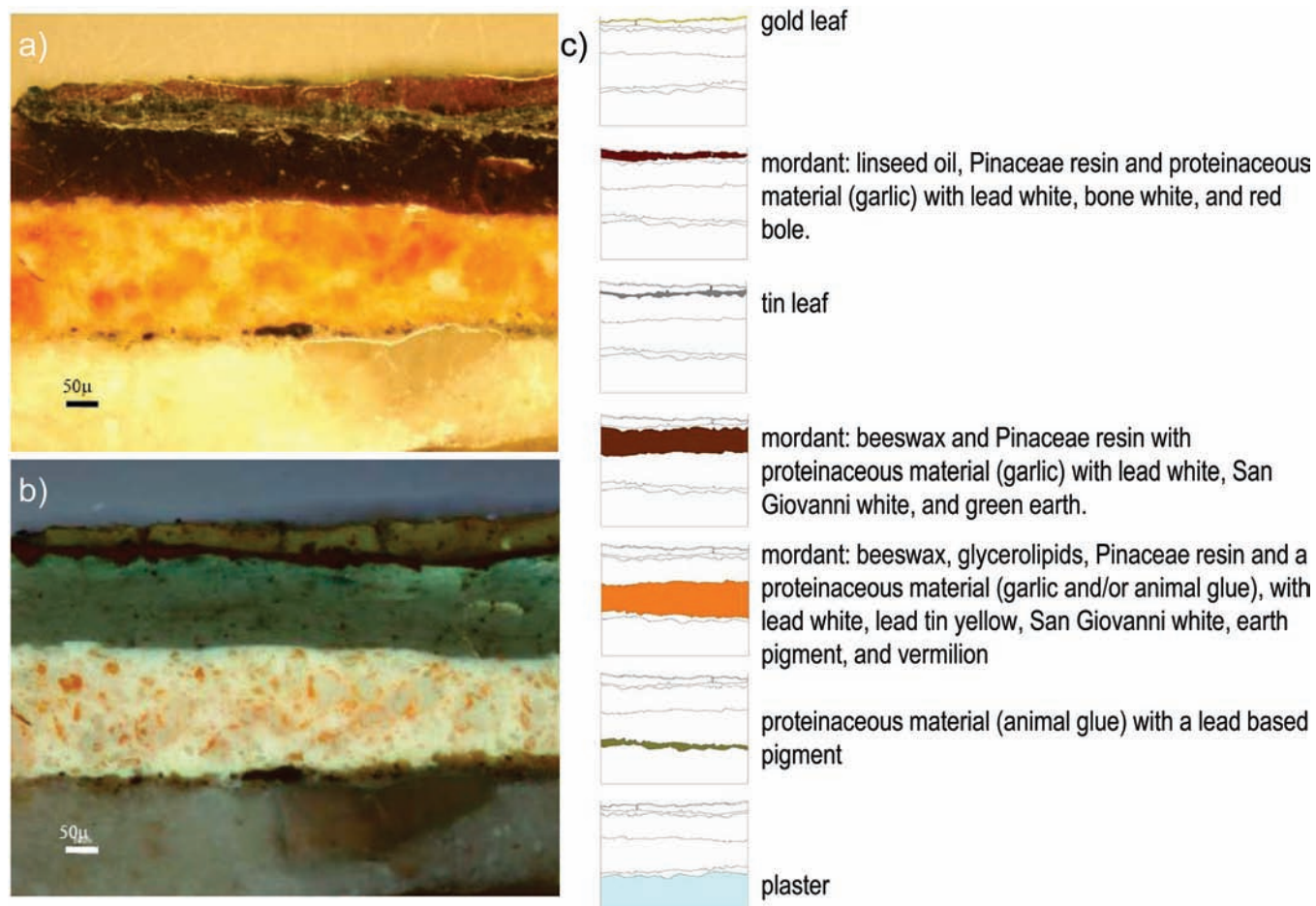
FIGURE 3. Sample collected from the gilding of the Orvetari Chapel: (a) cross-sectional image in dark field (white light); (b) same image in vis-fluorescence (UV light A filter); (c) sample composition, layer by layer. 10
