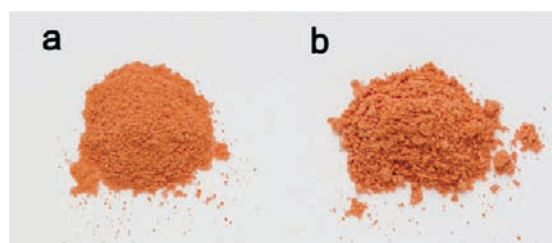
FIGURE 14. Yellowish red powder synthesized from iron containing glass and corundum: (a) as prepared; (b) heated at 1100 °C for 2 h in air.
