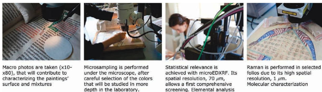
FIGURE 3. Main steps in a mission for the study of the medieval manuscripts from Alcobaca monastery (BNP, May 2009). MicroXRF and microRaman are techniques complementary to microspectrofluorimetry, that are used in situ . Microsamples will be afterward analyzed in laboratory, by microFTIR, microspectrofluorimetry, and microXRF. Photos by Duarte Belo.
