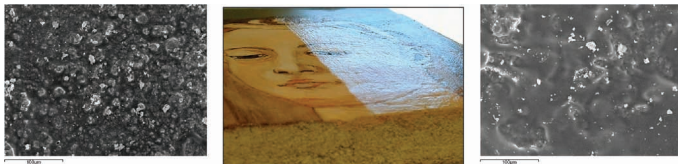
FIGURE 6. Mural painting sample treated, on the right side, with mowilith DM5 under glazing light (center), and SEM pictures of the uncoated (left) and coated (right) surface.
