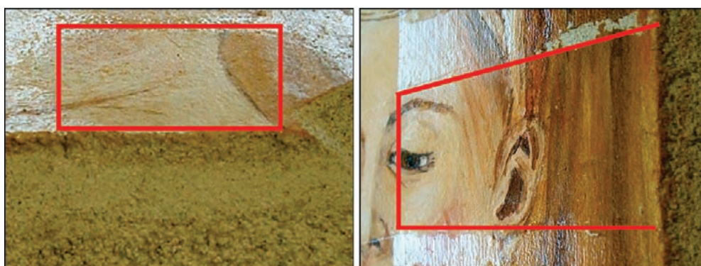
FIGURE 7. Details of the painting surface after removal of mowilith DM5 coating by using micellar solution (Mayapan system).
