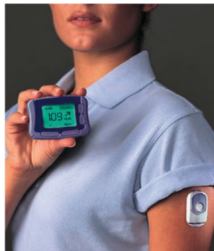
FIGURE 6. The FreeStyle Navigator system, the “wired” glucose oxidase-based, subcutaneously implanted continuous blood glucose monitor. The display shows a glycemia of 109 mg/dL; the directional arrow shows that the glycemia is increasing at a moderate rate. The sensor is implanted under the transmitter shown on the arm; the information is transmitted to and displayed by the hand-held display.
