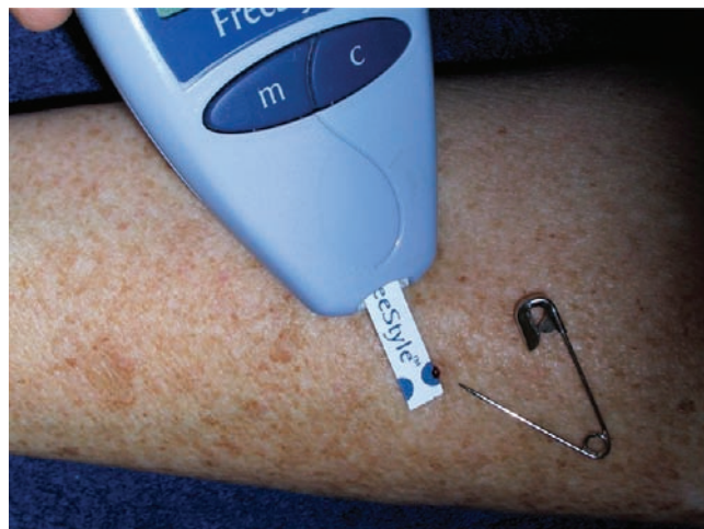
FIGURE 1. The FreeStyle microcoulometric strip and meter and a blood sample. The photograph is of the arm of Adam's wife, Ilana, taken in 2000.
