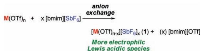
SCHEME 7. Proposed Anion Exchange between Metal Triflate and [bmim][SbF 6 ]
