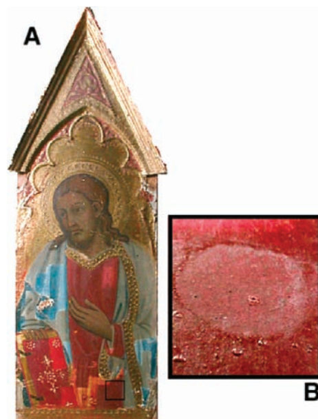
FIGURE 2. (A) A 16th century painting from the National Gallery in Siena, Italy. The black square defines the area where the cleaning test was conducted. (B) Grazing light image of the area treated with a 5 wt % PAA-CO 2 /1-pentanol gel. Reproduced with permission from ref 47. Copyright 2004 American Chemical Society.
