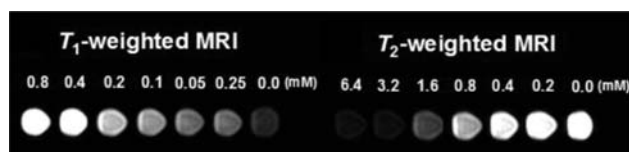
FIGURE 7. T_1 - and T_2 -weighted MRIs obtained from aqueous suspensions of Gd_8(OH)_{20}(H_2O)_{7.0} nanosheets. Reproduced with permission from ref 40. Copyright 2009 Royal Society of Chemistry.
