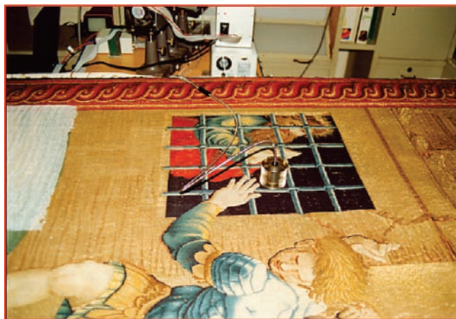
FIGURE 8. The portable fluorimeter at work on the tapestry Earthquake in Filippi .
