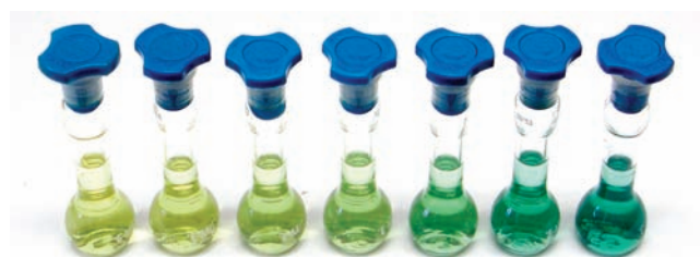
FIGURE 3. Solution of [\text{Pt}(\text{terpy})(\text{C}\equiv\text{C}-\text{C}\equiv\text{CH})]\text{OTf} (concentration = 1.47 \times 10^{-4} M) in acetonitrile–diethyl ether mixture demonstrating the remarkable color changes. Diethyl ether composition (from left to right): 64%, 68%, 72%, 74%, 76%, 78%, 80%.
