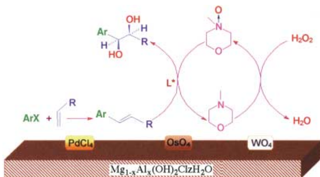
Scheme 1. The catalytic cycle in the LDH-PdOsW-catalyzed synthesis of chiral diols using H_2O_2 as the terminal oxidant.
