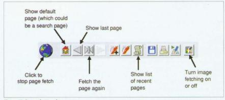
Figure III: Fresco button bar
