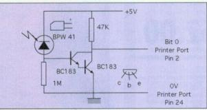
Figure I: An infrared receiver
