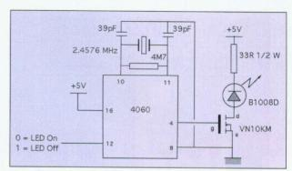
Figure IV: An alternative infrared transmitter circuit
