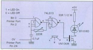
Figure III: The infrared transmitter circuit
