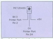
Figure II: An alternative infrared receiver
