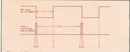
Figure 2. Timing diagram for versatile interface adaptor pulse generator. T1 is set by timer 1 and T2 is set by timer 2
