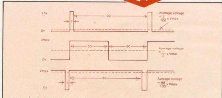
Figure 1. Variable mark-space ratio pulses producing different average voltages
