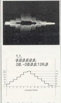
Figure 4. Variation in amplitude controlled by the envelope statement. Oscilloscope trace starts on the third increment
