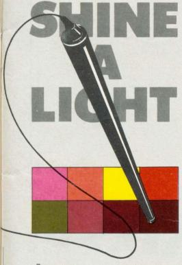
A typical lightpen picks up light given out by the TV screen. The pen sends an electronic signal into the micro, where circuitry decodes the position on the screen at which the pen is pointing. Software can access this input, tailor it to the screen mode and allow the user to play games, draw and 'paint'. design layouts, select multiple choice answers, update and alter information using a menu, or interact with graphic simulations. And these are just a few applications.
