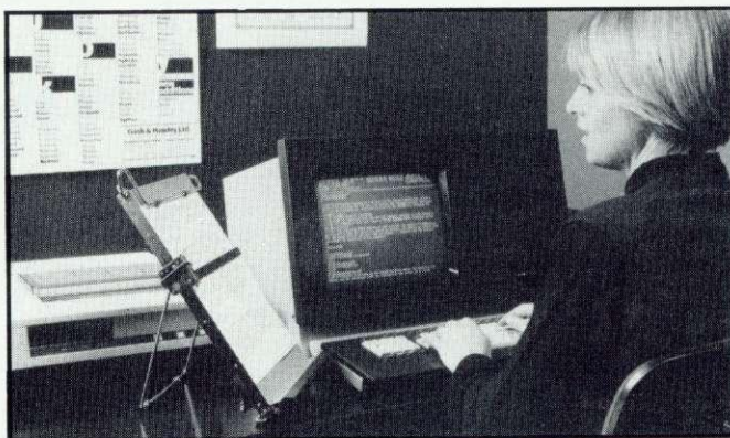
Torch with modified keyboard and running Cora 5, a language devised for the Linotron typesetters
