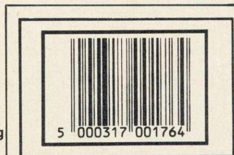
Figure 3. Typical barcode label using the EAN13 system
