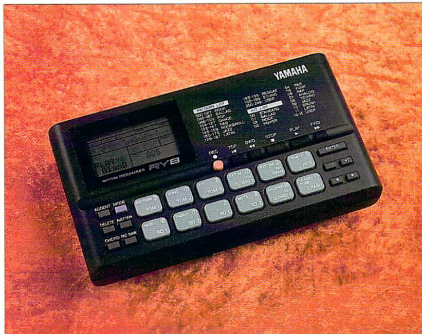
Recording rhythm patterns from this Yamaha RY8 drum machine is a prime candidate for using your sequencer's external clock option
