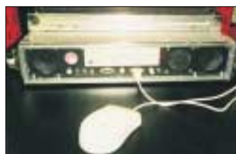
Above: An Eyetech A1200 special. This 19" rack mount is intended for multimedia presentations. There is also a version that uses a small ROM in place of the floppy drive to enable it to boot from a CD-ROM.
