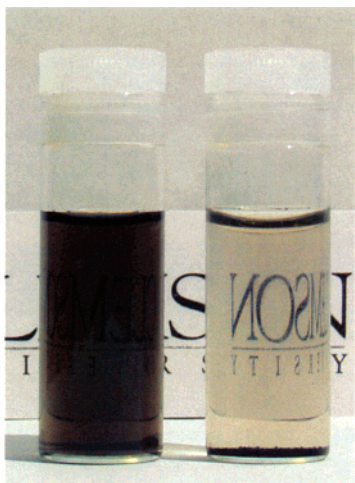
Figure 1. Visual comparison of the supernatants from centrifuging the aqueous dispersions of Gal 2 -MWNT (left) and Gal-MWNT (right).
