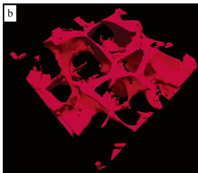
Figure 2. (a) A single X-ray microcomputed tomography slice showing the porous interior of an EBPADMA-300 scaffold and (b) a 3D compilation of 100 slices of the X-ray micrographs.
