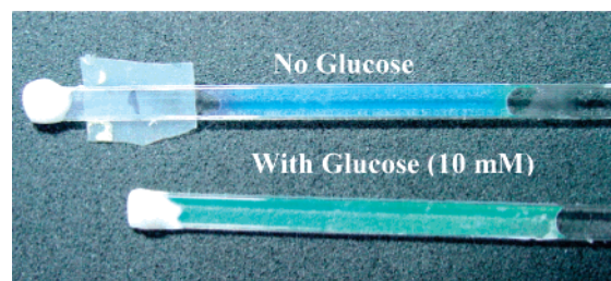
Figure 13. Photograph of the rectangular capillaries filled with the colloidal crystals composed of 5% APBA microgels without glucose and in the presence of glucose (10 mM) in Tris (2 mM), pH 8.5.
