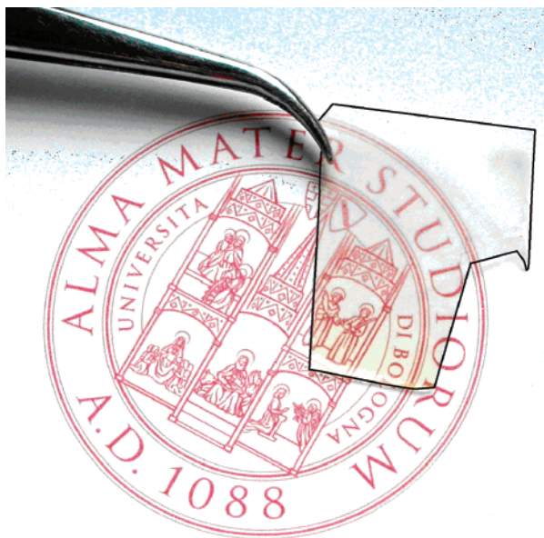
Figure 6. Transparent A50-130 film (0.25 mm thick). The hybrid sample shape is outlined by the black line for the sake of easy location.
