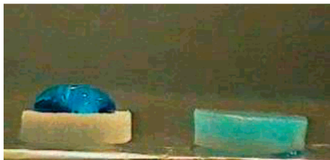
Figure 1. HYAFF11 (left) and HYAFF11 autoloading (right) sponges, demonstrating the effect of hydrophilic HA coating of HYAFF11.
