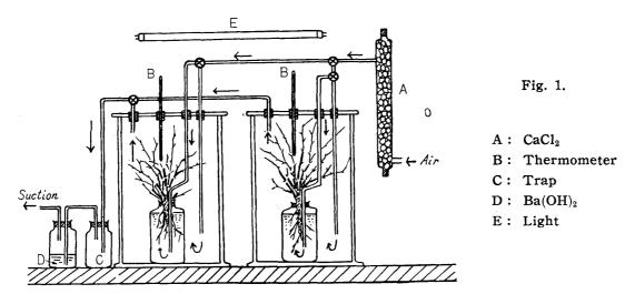
The outlet tubing was connected to a trap bottle containing  $Ba(OH)_2$  solution to hold radioactive  $CO_2$  generated from the plant, whose radioactivity became detectable from the 3rd day of cultivation. The temperature range recorded during the cultivation was  $20 \sim 30^{\circ}$ .
