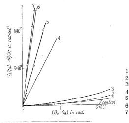
Fig. 1. Initial Rate vs. Angular Twist for Different Rancidity Peanut Oil-Aluminum Stearate Gel (2% w/v)  $K_2 = 58 \text{ dyn.cm}.$
