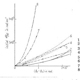
Fig. 2. Initial Rate vs. Angular Twist for Various Oil and Aluminum Stearate Gel (2% w/v)  $K_1 = 273 \ dyne/cm$ .
