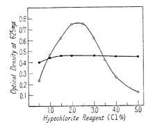
Fig. 3. Effect of the Concentration of Hypochlorite Reagent on the Color Development
