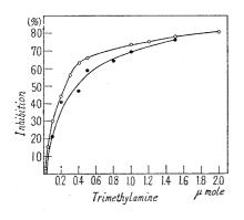
Fig. 1. Relationship between Amount of Trimethylamine and its Inhibition of Color Development
