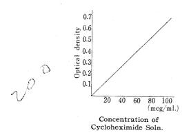
Fig. 5. Standard Curve for Spectrophotometric Determination of Cycloheximide
