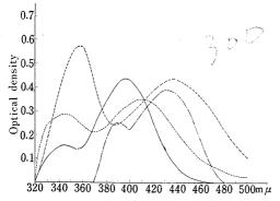
Fig. 1. Absorption Spectra shown by Cycloheximide when heated with Various Resorcinols in Hydrochloric Acid
