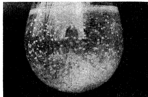
(B): after 3 hrs.; Particle size of sulfathiazole is apparently enlarged by the accumulation of the molecular compound formed.
