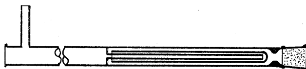
Fig. 2. Diagram of Kashiwagi's Combustion Tube
