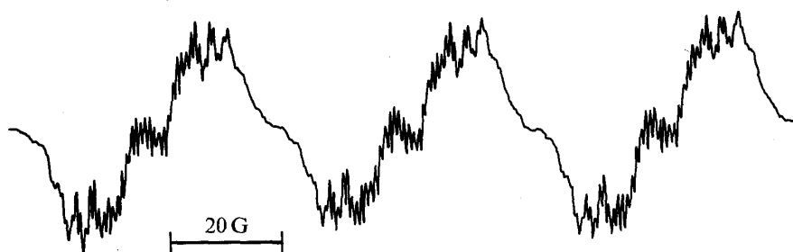
Fig. 4. ESR Spectrum of an in Situ Electrolyzed Solution of the Nitrosamine 3 (10 mM) in Propionitrile (0.1 M \text{NaClO}_4 ) at -70^{\circ}\text{C}
