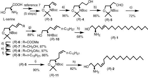
Reagents and conditions: a) i) 9-BBN, THF, rt, 12 h; ii)  $H_2O_2$ , NaOH, rt, 4 h, b) Dess-Martin periodinane,  $CH_2Cl_2$ , rt, 0.3 h, c)  $Ph_3P=CHCO_2Me$ , PhMe, reflux, 0.5 h, d) DIBAH, THF, -78°C, 10 h, e) Ac<sub>2</sub>O, pyridine, rt, 12.5 h, f)  $n-C_12H_25MgBr$ ,  $Li_2CuCl_4$ , THF, -15~0°C, 5 h, g) Amberlyst-15, MeOH, rt, 26 h, h) c.HCl, AcOEt, rt, 22 h for (R)-10, 1 h for (R)-11, i)  $n-C_14H_29P+Ph_3$   $Br^-$ , n-BuLi, THF, rt, 2.5 h.
