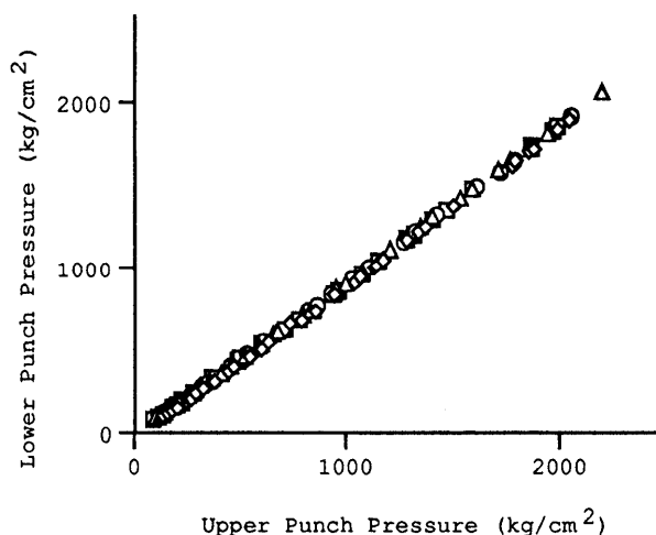
Fig. 6. Compression Pressure Plot of Upper Punch vs. Lower Punch
