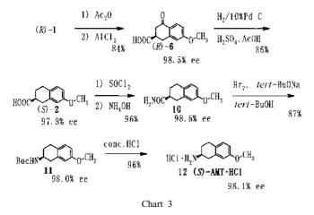
treated with concentrated hydrochloric acid (conc. HCl) to give (S)-AMT·HCl (12) in 96% yield with 98.1% ee (Chart 3).
