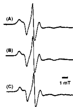
Fig. 2. ESR Spectra of EPC/5-DS SUV at Re=0 (A), 0.15 (B), and 0.20 (C) at 28 °C
