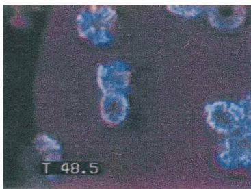
Fig. 6. Photo Micrographs of PEG 6000 during Crystallization (Magnification: \times 100 )
