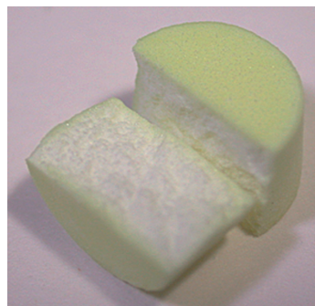
Fig. 2. Extreme Case of Drug Migration Caused by Excess Ethanol (Actual Photograph)
