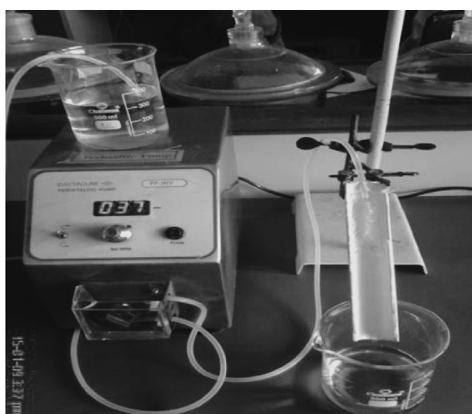
Fig. 6. Test Apparatus Designed for in Vitro Mucoadhesive Strength Determination of Microspheres
