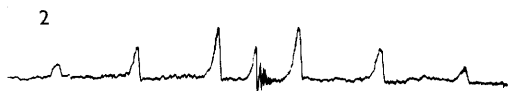
FIG. 2. The spectrum of trimethyl phosphite and a sideband (678 c./sec.) from a capillary of P_4O_6 (bore approximately 1.5 mm.), showing the narrower line from the latter compound.
