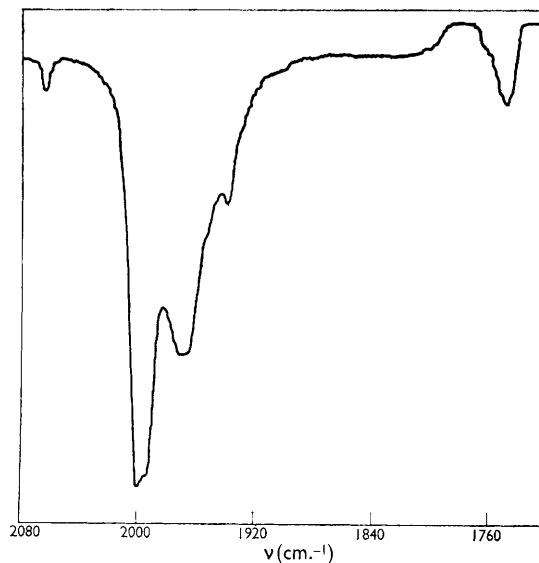
FIGURE 2. Infrared spectrum of [\text{Et}_3\text{NH}]^+[\text{HFe}_3(\text{CO})_{11}]^- in tetrahydrofuran; 0.46 mg./ml.
