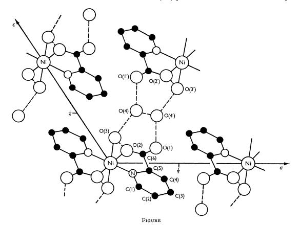
Intensity data were recorded on multiple-film Weissenberg photographs for a cylindrical crystal of 0·3 mm. diameter rotating around the b-axis (Cu- $K_{\alpha}$ : $\lambda = 1.5418$  Å; 772 non-zero reflexions).
