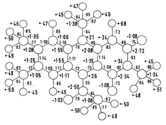
FIGURE 3. Calculated net charges (values with signs) and overlap populations. All values are given in electron units.
