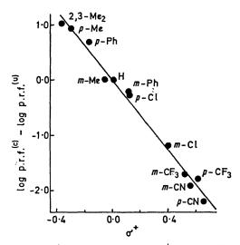
Hammett plot:  $\sigma_p^+$  for 1-position and  $\sigma_m^+$  for 4-position:  $\sigma_p^+$ -me +  $\sigma_m^{+-}$ -me for 2,3-dimethylbutadiene (designated by 2,3-Me).
