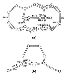
FIGURE. Experimental geometry of the carbon skeleton of 1,6:8,13butanediylidene[14]annulene. (a) Bond lengths, angles, and (in parentheses) torsion angles. (b) Dihedral angles.
